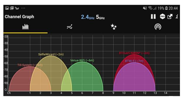
However, due to the way the Channels overlap this could potentially result in interference from the Till System running on Channel 1 and the Venue Wi-Fi on Channel 6.
